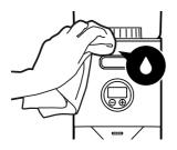
Use a soft cloth, preferably microfiber, like the Lelit cloth (code MC972 - not included), and moisten it with plain water. Do not use abrasive detergents and do not immerse the grinder in water.
